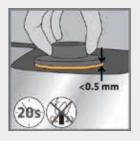
Bonding needs WET on WET. Hold for approx. 20 seconds. Excess material can be removed
