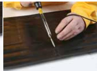
Strengthening with welding strip using welding tip
