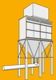
Sealing and bonding of metal sheets in air treatment and ventilation systems with Sikaflex®-522 for ultimate mold and fungus-resistance.
