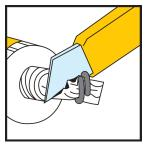
2. Cut the end off the protective film
